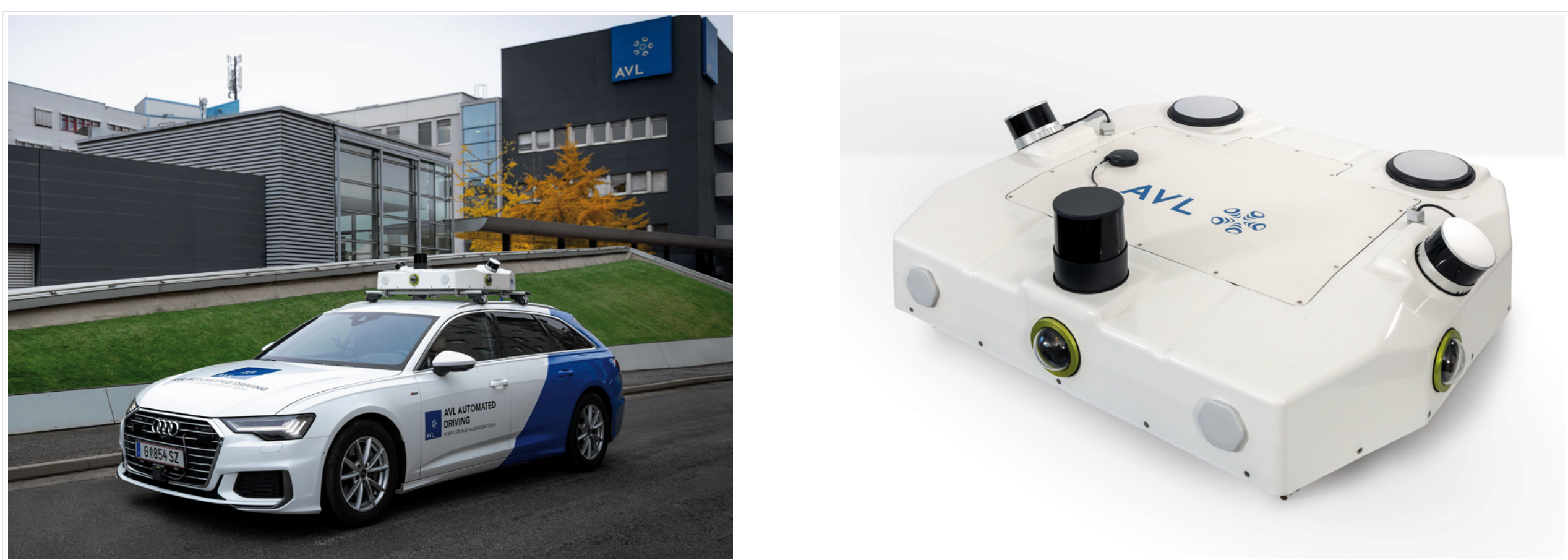
Figure 1: Knowledge gap demonstrator setup (left: DGT system mounted on top of a test vehicle, right: close-up of the DGT system) (© AVL Deutschland GmbH)
